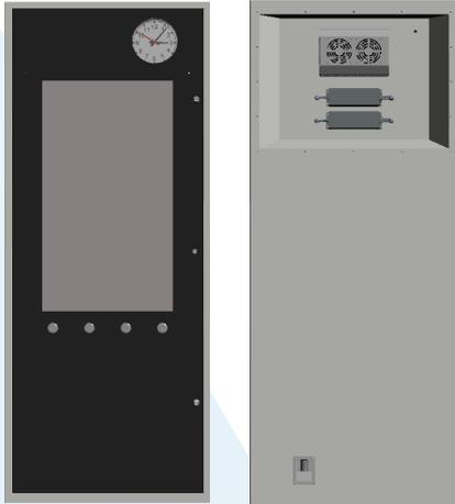
The device is part of the Dynamic Passenger Information System (SDIP) used to provide up-to-date information on train arrivals and departures at a given station. The interactive kiosk is built around a professional-grade 46" Full HD screen capable of prolonged operation in a wide range of temperatures. The design is adapted to long-term operation in a wide range of temperatures.
