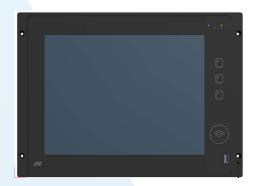
Operator panel with a 15" display. Designed for use in railway vehicles. Housing with function buttons and optical sensor that automatically adapts the brightness of the display to the prevailing lighting conditions. The device is also equipped with USB ports and an RFID reader; selected models are also equipped with a touch overlay on the screen.
